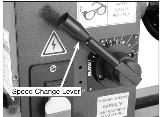
Figure 9. Speed change lever.
